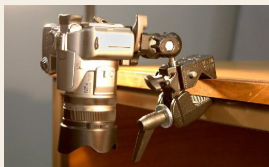
Example of a camera clamp in use. Image courtesy of Andrew Long, Coffs Harbour City Council
