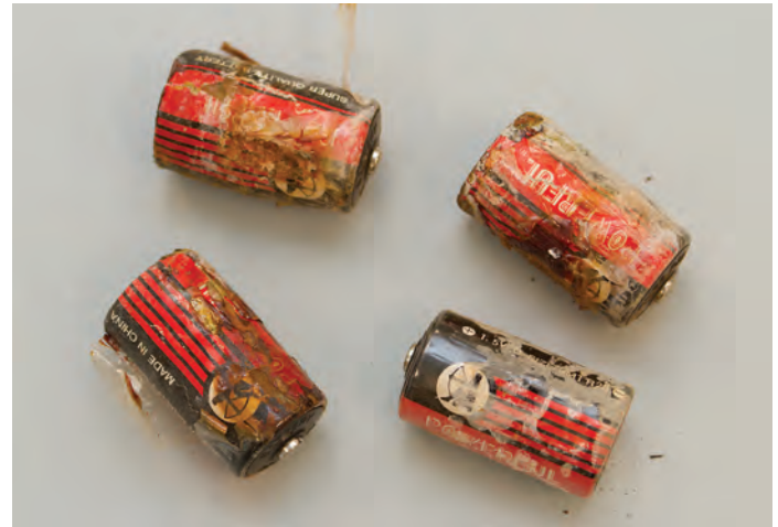
The battery acid in these metal and plastic batteries has caused them to degrade.
