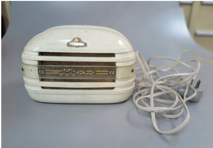
Formaldehyde plastic (white bakelite) from this 1947 Astor mantle radio is extremely sensitive to water.
